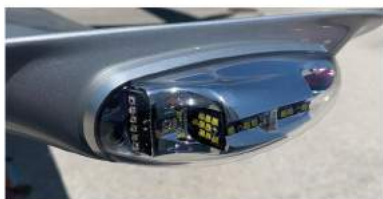
CIRRUS ORION 600 LED SR-20 SR-22 WINGTIP CONVERSION
