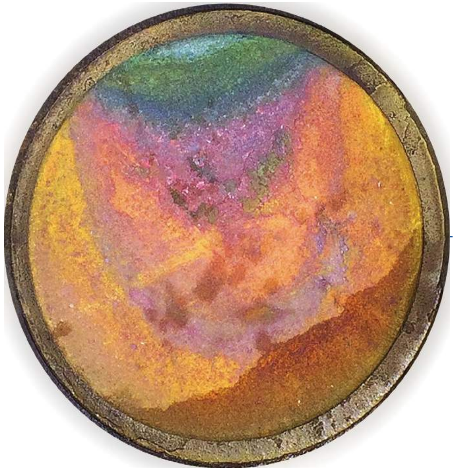
⤴ A burned exhaust valve.
